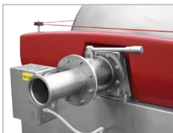
overfilling signalisation, axial filling valve
