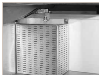
strainer on the pan outlet
