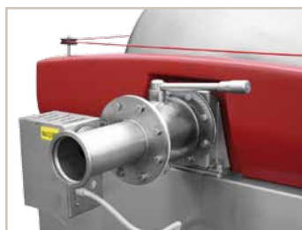
overfilling signalisation, axial filling valve
