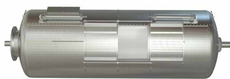
double sliding hatch with pneumatic drive
